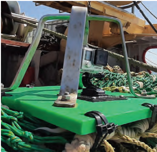
Figure 2. Impression of camera set-up positioned on the upper side of the cod-end prior to setting the flyshoot trawl net. (Photo credit: P. Molenaar)
