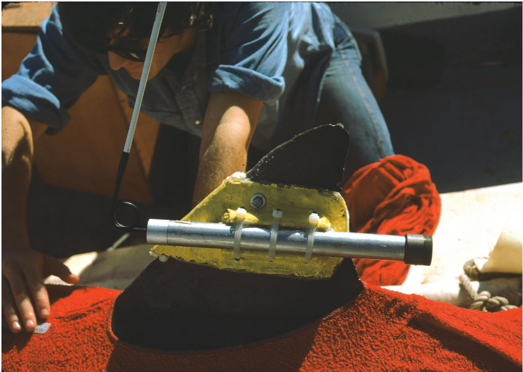
Figure 19. Michael Scott hovers behind a radio tag attached to a fiberglass saddle bolted through the dorsal fin of RT-1. The spring antenna design maximized chances it would reach the surface to transmit each time the dolphin took a breath. The antenna was moved aft and made more flexible on subsequent radio iterations.
