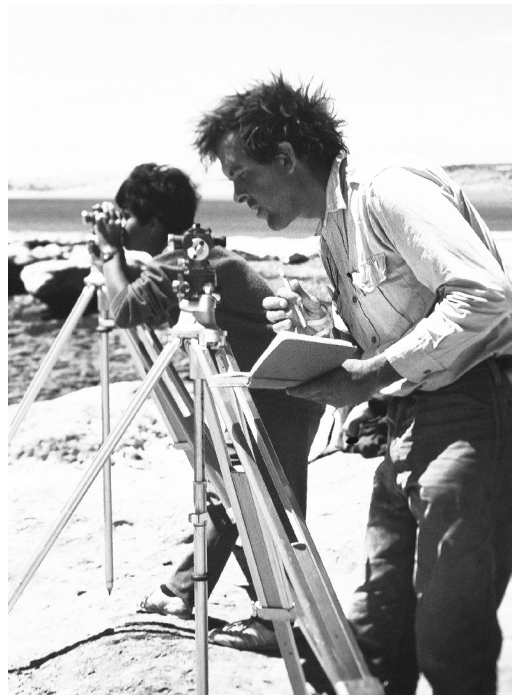
Figure 8. Roger Payne and Melany Würsig "duel with" two Kern DKM theodolites to inter-calibrate them for increased accuracy, November 1974 (Photo courtesy of B. Würsig)
