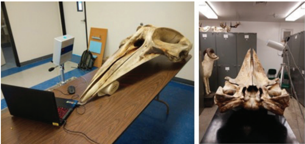
Figure 1. Photos of minke whale ( Balaenoptera acutorostrata ) specimens to illustrate use of the 3D laser scanner and 3D model obtained
