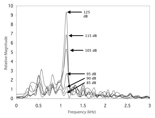
Figure 3. Fast Fourier transform (FFT) of the waveforms from Figure 2; the FFT response magnitudes are a relative measure of the acquired waveforms. Note the decreasing amplitude of the FFT with decreasing stimulus amplitude.
