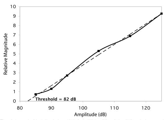
Figure 4. An example of threshold evaluation at 16 kHz for the FFT data of Figure 3; the solid line and points are actual measured data points, and the checked line is a linear regression line, which, when the zero point is calculated, assigns the threshold for this frequency at 82 dB.
