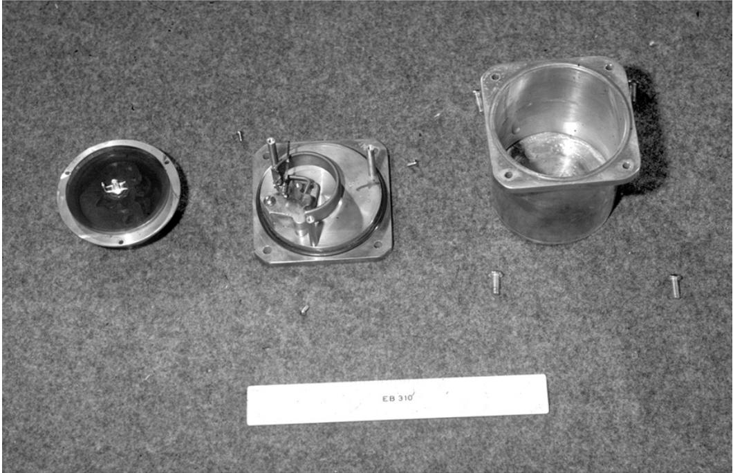
**Figure 7.** The first TDR designed and deployed on a diving animal; the casing is brass, and the kitchen timer is under the mounted smoked glass on the left.
