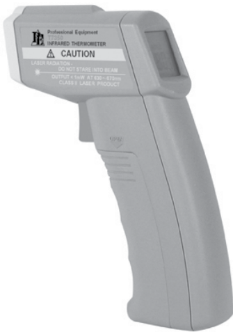
Figure 1. Professional Equipment T7350 Series Infrared Thermometer used to take surface temperatures of the torso and flippers of the California sea lions and of the water and land substrate on- and off-exhibit at the Peoria Zoo
