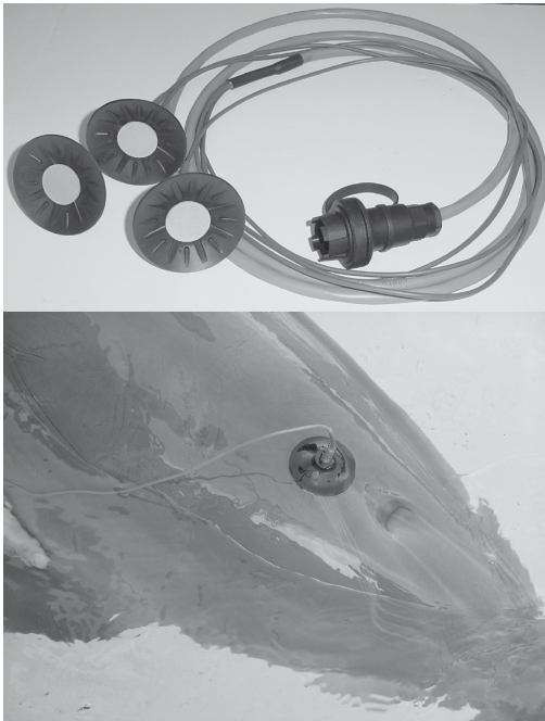
Figure 9. OdiSEA's electrodes with 3-m cable and IP68 connector (top); signal electrode positioned 10 cm behind Isaac's blowhole (bottom).
