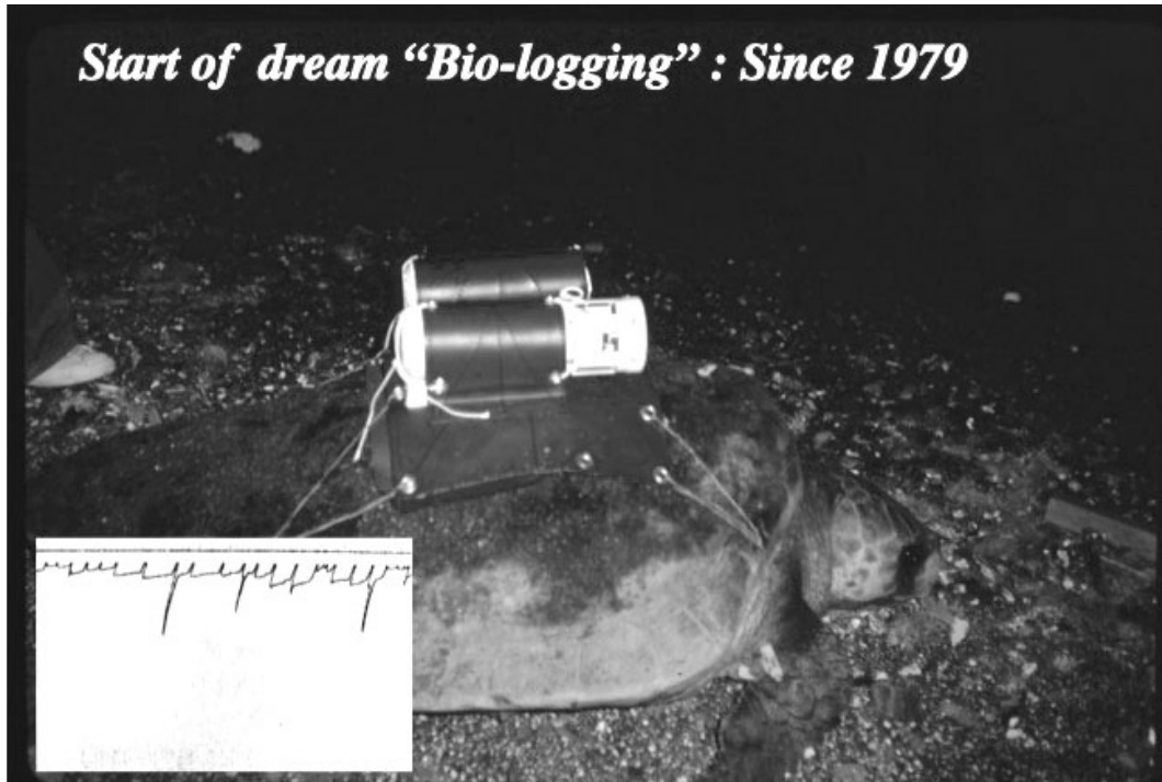
Figure 2. At an early stage of development of the time-depth recorder (TDR) and swim-speed recorder (SSR), I used a fishing net recorder, which only turtles were able to carry. Our TDRs recorded depth in arc form, requiring a conversion protocol using a digitizer. Following these experiments, the miniaturization of ABDs was my primary objective.
