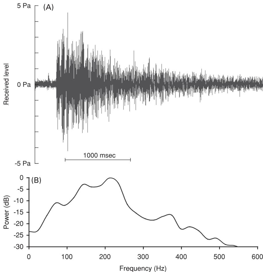
**Figure 2.** (A) Waveform of a sleeve air gun pulse. (B) Power-spectrum of the pulse from Figure 2A. FFT-size=2048.
